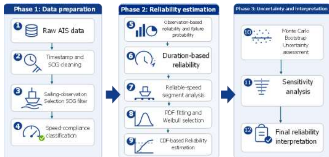
Figure 1. Analytical Workflow for Processing AIS Data and Estimating Service-Speed Reliability
